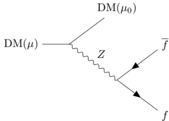
$$\text{Decay width} \sim \frac{g_Z^4 \sin^4 \alpha \mu_0^5}{m_Z^4} \times \left( \frac{\Delta\mu}{\mu_0} \right)^{13/2} \quad (\text{w/ } \Delta\mu = \mu - \mu_0)$$
